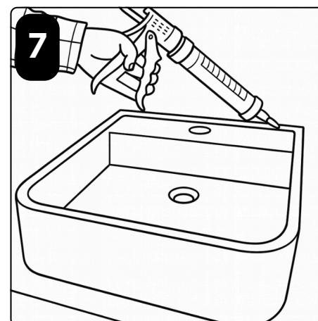
APPLY SILICONE TO SURFACE OF SINK THAT IS TOUCHING THE WALL; USE PAINTER'S TAPE TO ASSIST WITH CLEAN LINES
