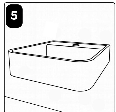
CAREFULLY PLACE SINK IN ITS INTENDED LOCATION, ALIGNING SINK OVER BRACKETS CENTER
