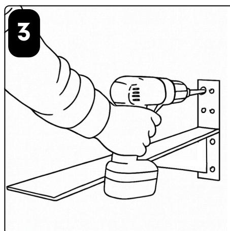
USE CONSTRUCTION SCREWS TO SECURE BRACKET TO CHOSEN BACKING. ENSURE THAT BRACKETS ARE LEVEL TO EACHOTHER
