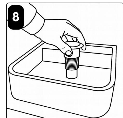
FILL DRAIN AREA WITH PLUMBERS PUTTY SURROUNDING DRAIN RIM, SLIDE DRAIN INTO PLACE, HAND-TIGHTEN. **DO NOT OVER TIGHTEN**
