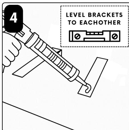
INSTALL DRYWALL OVER THE BRACKETS AND APPLY SILICONE TO TOP OF BRACKETS
