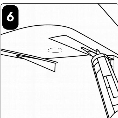
APPLY SILICONE TO UNDERSIDE OF SINK, SEALING TO THE PERIMETER OF BRACKETS
