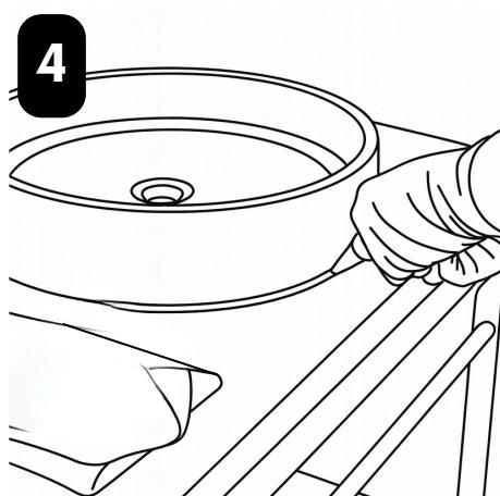
RUN A BEAD OF CLEAR BATHROOM SILICONE TO SECURE THE BASIN TO THE COUNTER
