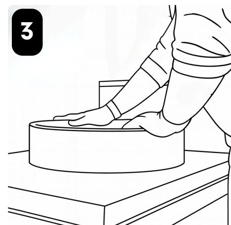
PRESS DOWN INTO COUNTER AND REMOVE EXCESS SILICONE USING DENATURED ALCOHOL AND CLOTH
