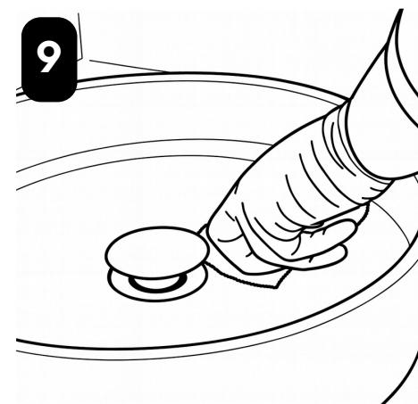
REMOVE EXCESS PUTTY, ALLOW SILICONE TO DRY FOR 24 HOURS BEFORE USE
