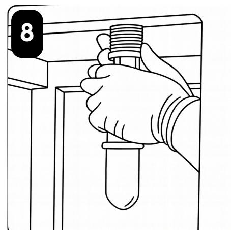
SLIDE DRAIN INTO PLACE, HAND-TIGHTEN. DO NOT OVER TIGHTEN
