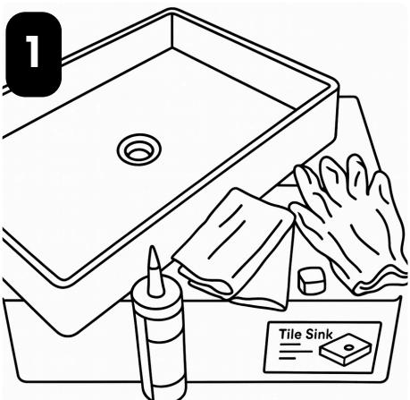
REMOVE SINK FROM BOX AND PUT IN INTENDED SPACE. GATHER GLOVES, BATHROOM SILICONE, CLEAN CLOTHS, AND DRAIN ASSEMBLY
