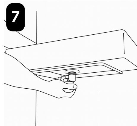
SLIDE DRAIN INTO PLACE, HAND-TIGHTEN. DO NOT OVER TIGHTEN
