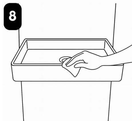
REMOVE EXCESS PUTTY, ALLOW SILICONE TO DRY FOR 24 HOURS BEFORE USE
