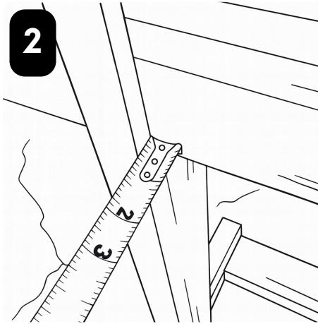
INSTALL A CROSS MEMBER BETWEEN STUDS, RECESSED 1/4" FROM FLUSH FACE OF STUD.
