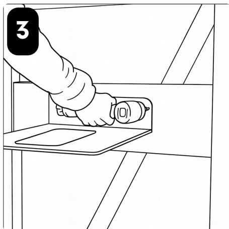
USE MINIMUM 4 HOLES TO SECURE BRACKET TO CHOSEN BACKING.
