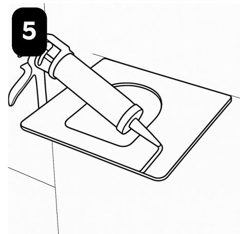
APPLY SILICONE TO TOP OF BRACKET. THEN CAREFULLY PLACE SINK IN ITS INTENDED LOCATION, ALIGNING SINK OVER BRACKET CENTER.
